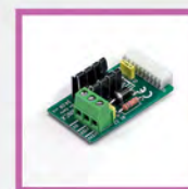
DA.RB 9760042 Battery charger card for DA.S04.
