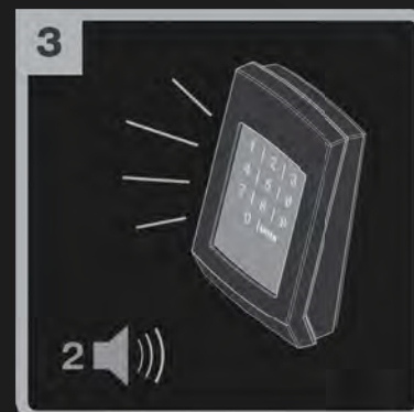
3 Two beeps and two flashes of the back lights indicate the completion of transmission
